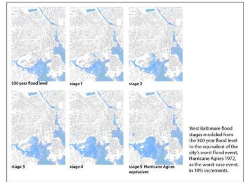
Figure 7. Flood risk stages for West Baltimore, 500 year flood base with 10% incremental increases to Hurricane Agnes level, the worst flood in Baltimore’s history. Source: O’Meara, K., & Kim, E. (2016). HIGHER GROUND: Leveraging Baltimore’s Topography to Increase Social and Climate Resiliency through Landscape.
